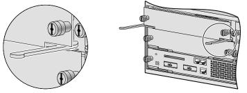
3. With the line card halfway out of the slot, disconnect all cables from the line card. After disconnecting the cables, pull the line card out of the chassis slot.
